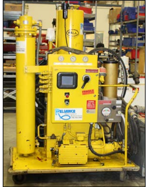
The HVP Purifier is mounted on castors for easy mobility.
